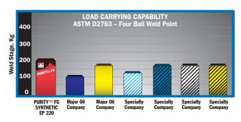
PURITY FG SYNTHETIC EP Gear Fluids also provide higher load carrying capability than many major oil companies' and specialty lubricant suppliers' gear fluids, so it's ideal for food processing applications running under heavier loads.
